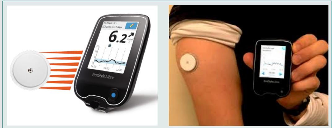
Figure 1. The FreeStyle Libre Flash Glucose Monitoring System (Abbott, Diabetes Care, Alameda, California, USA), and the sensor and reader in use.
